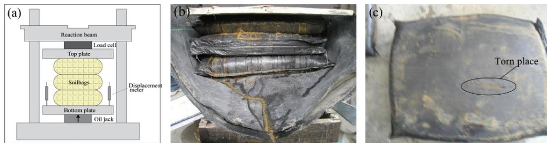
Fig. 1. Unconfined compression tests on clay-filled soilbags: (a) Schematic view; (b) Under compression; (c) Torn place on the soilbag surface.
