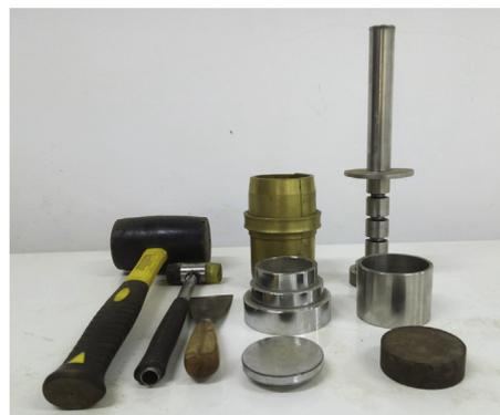
Fig. 3. The device for compacting expansive soil specimen.
