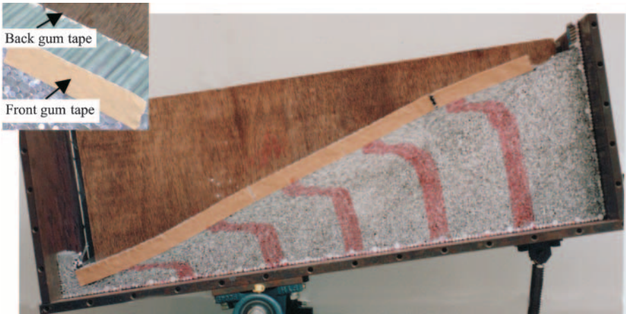
Fig. 15. Photo at failure: 10 strips of gum tape (15 cm × 2.5 cm) were pasted on the front and back faces of the slope along the descendent slope direction; no restraint at the slope toe.
