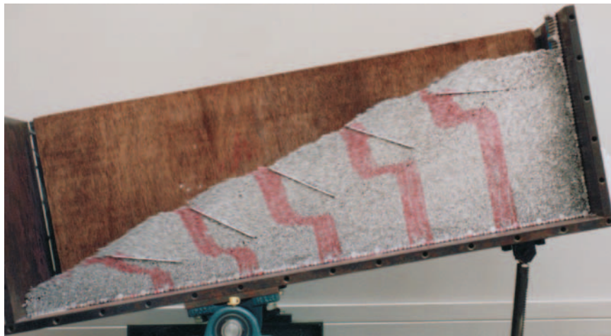
Fig. 14. Photo at failure: five pieces of thin aluminum sheets, simulating soil nails, were inserted along the \sigma_3 direction (insert depth, 10 cm).
