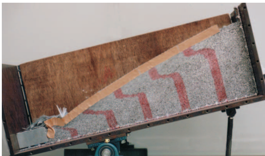
Fig. 16. Photo at failure: 10 strips of gum tape (15 cm × 2.5 cm) were pasted on the front and back faces of the slope along the descendent slope direction. A thick block was installed at the slope toe acting as a retaining wall.
